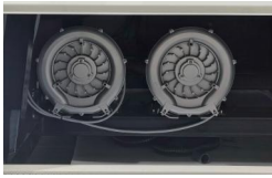
The new two high-power 1.5kw suction motors, with six suction areas, increase the suction power, and the old one 1.5kw motor is not easy to suck
