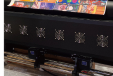
Three stage heating system including pre-heater, print heater, and rear heater and platform vacuum system with adjustable
