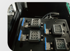
Automatic moisturizing function to extend the life of the heads
